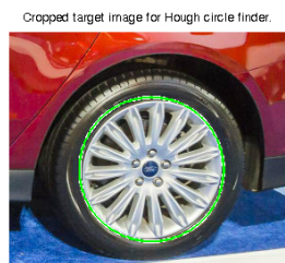
Figure 17. Successful Hough ellipse match to rear wheel (match highlighted in green).
