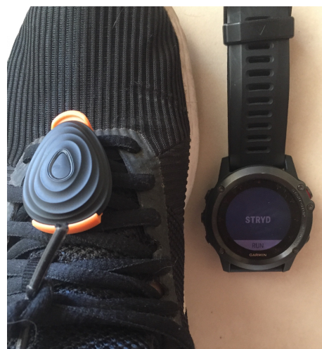
Figure 2. The dependent variable power output is measured with the Stryd sensor and recorded on a Garmin watch.
