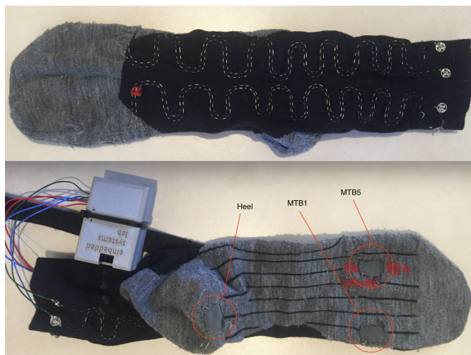
Figure 1. Smart socks with sensors and data acquisition unit provide the independent variables for the analysis.
