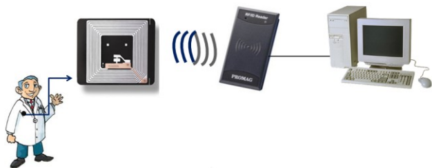
Figure 2. RFID system (reader+tag)
