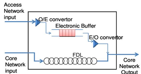
Figure 2. Architecture of Hub
