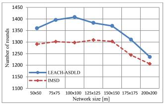
Figure 2. LEACH-ASDLD half nodes die vs. IMSD last node dies.
