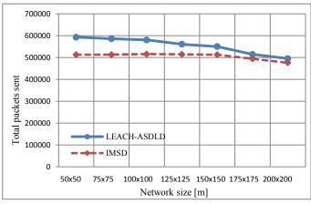
Figure 3. LEACH-ASDLD vs. IMSD – total number of packets sent for different network sizes
