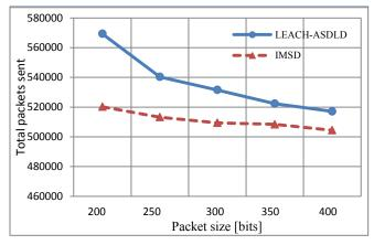
Figure 5. LEACH-ASDLD vs. IMSD – total number of packets sent for different packet sizes
