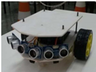
Figure 1. Structure Generic Robot using Arduino Mega
