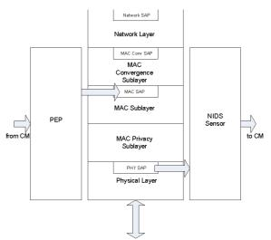
Figure 2. Protocol stack of IPS in HAP 802.16 network. CM is correlation module.
