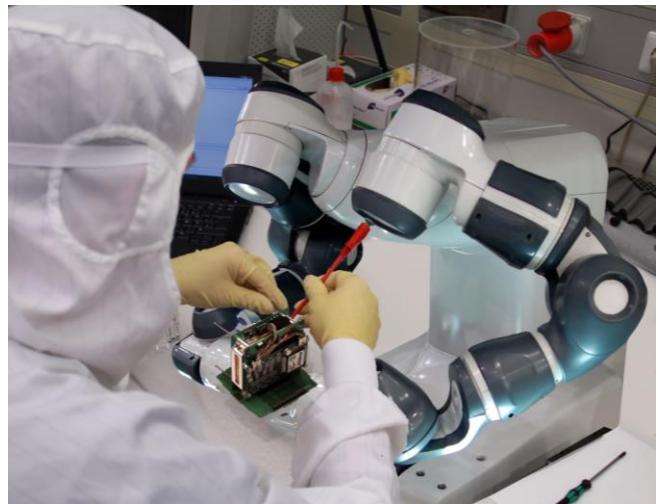
Figure 4. Human-cooperation at Zentrum for Telematics, Würzburg, to jointly integrate and test satellites. The robot acts as a third arm and contributes high precision motion capabilities.
