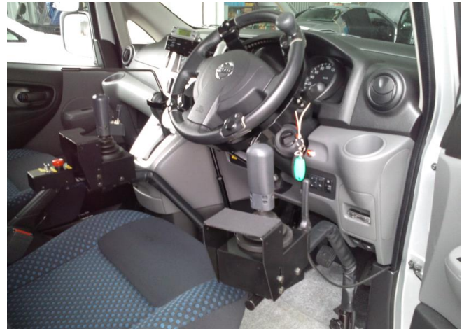
Figure 2. Wada and Kameda's joystick driving interface
