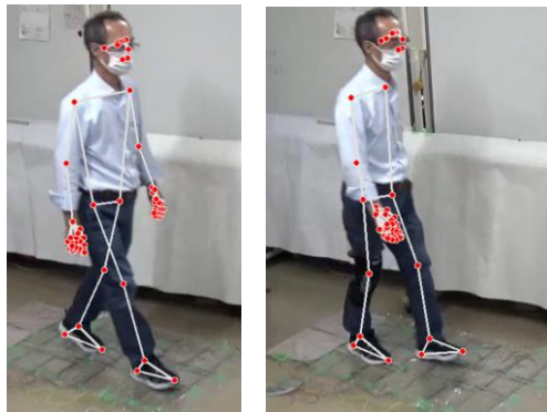
Figure 5. Skeleton analysis of motion (a) without and (b) with restrictions using video from oblique upward angle.
