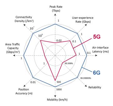
Fig. 3. Comparison between 5G and 6G requirements [21]
