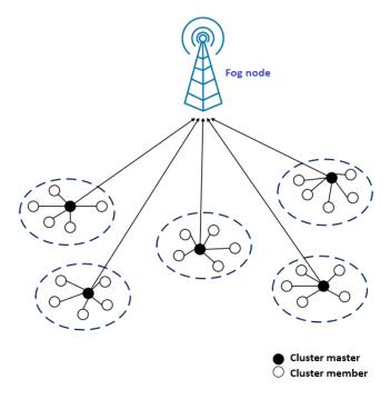
Fig. 5. Clustered Architecture to Fog Network [34]
