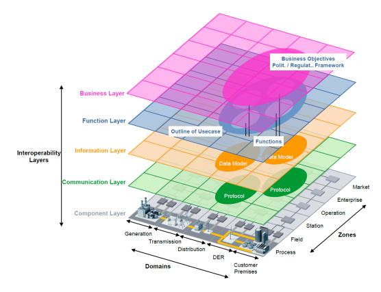
Figure 1. M/490 Smart Grid Architecture Model [5]
