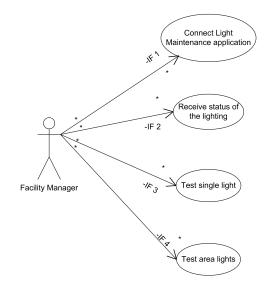
Figure 2. ROFCO Use Case Light Maintenance
