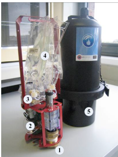
Figure 1: GEN2 Nutrient analyzer design; (1) Sample inlet; (2) Control board and detection system; (3) Dual channel peristaltic pumps; (4) Reagent bags; (5) IP68 enclosure
