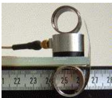
Figure 6. AE sensor is fixed with a spring instead of the dead weight used for the tests.
