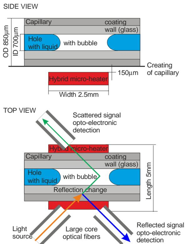
Figure 1. Schematic construction of the capillary head.
