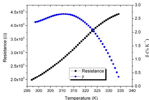
Figure 2. Sample's electrical resistance and  $\beta$  versus temperature
