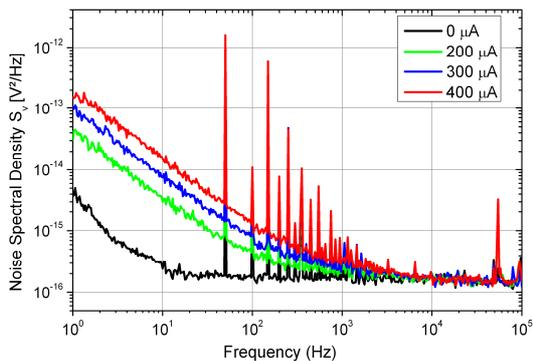
Figure 5. Noise spectral density measured in the four probe configuration at different bias currents at 318K.
