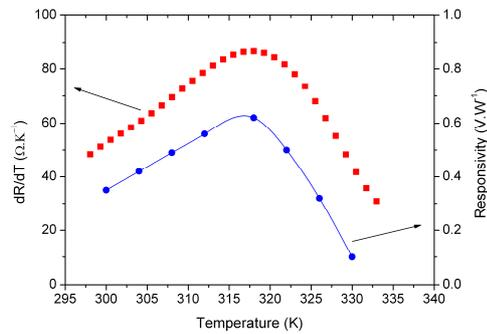
Figure 3. Optical responsivity  $\mathfrak{R}_v$ , at bias current  $400 \mu\text{A}$  and frequency 1 Hz and  $dR/dT$  versus temperature curves.
