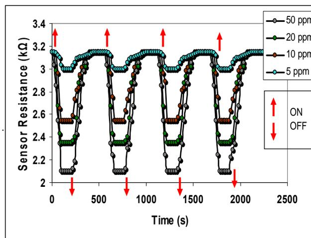
Figure 10. Dynamic response of the sensor for different concentration of methanol vapors at operating temperature of 50 °C. The arrows indicate the switching ON and OFF of N<sub>2</sub> flowing through the bubbler containing methanol.
