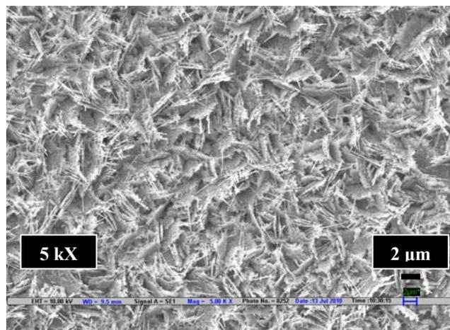
Figure 7. SEM image of ZnO nanocombs obtained after annealing Zn film (300 nm) at 300 °C for 12 h.
