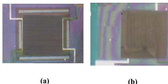
Figure 5. Optical photograph of sensor fabricated on (a) diaphragm (2 μm) and (b) using thermally isolated platform technology.
