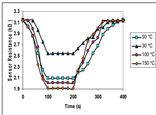
Figure 8. Response of the sensor to 50 ppm of methanol vapors at different operating temperatures.
