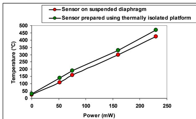
Figure 6. Power versus temperature plot of microheater fabricated on suspended diaphragm (2 μm) and sensor fabricated using thermally isolated platform technology.
