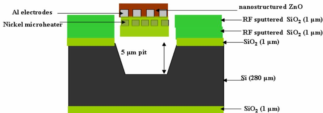
Figure 1. A schematic diagram of the MEMS gas sensor on a suspended platform.
