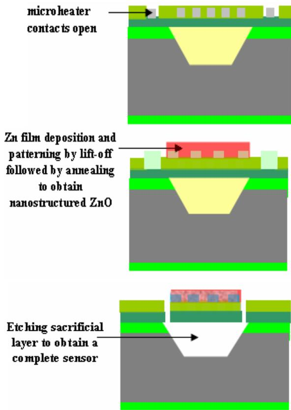
Figure 2. Process flowchart of sensor fabricated on suspended diaphragm.
