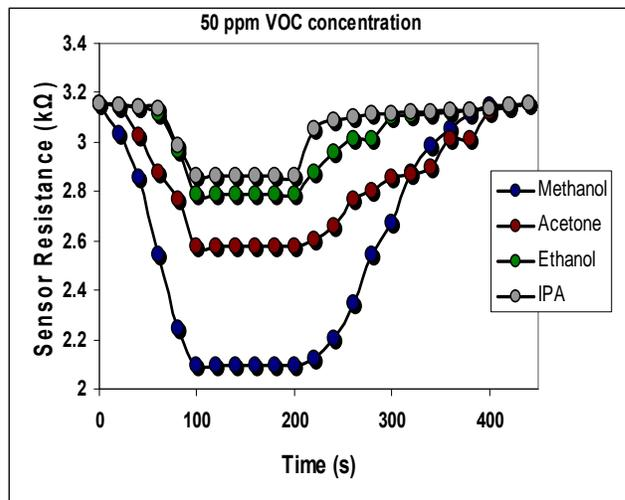
Figure 9. Response of the sensor to different VOCs at 50 °C operating temperature.
