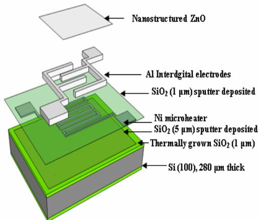
Figure 3. Blown-up diagram of the sensor fabricated on thermally isolated planar platform.
