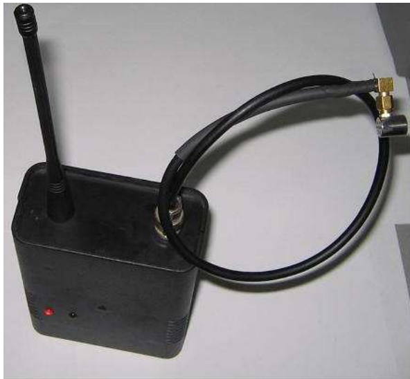
Figure 5. Experimental wireless module for acoustic emission sensor.
