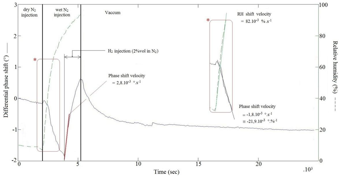
Fig. 5. Influence of humidity on the detection of hydrogen at constant room temperature ( $19.3 \pm 0.1^\circ\text{C}$ ).
