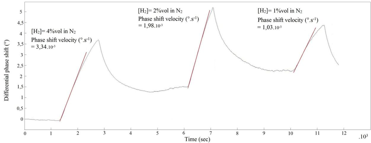
Fig. 4. Detection of hydrogen in the range 4% to 1%vol in N<sub>2</sub>.
