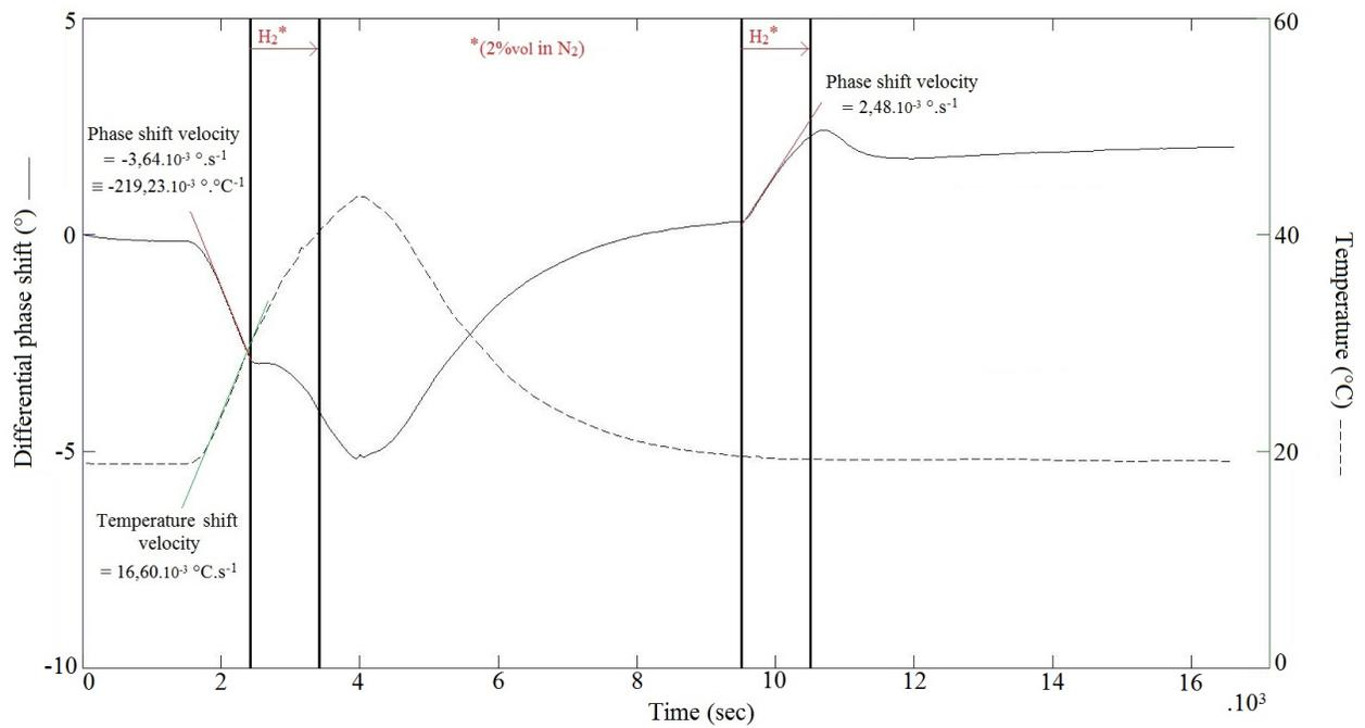
Fig. 6. Influence of temperature on the detection of hydrogen (RH in the 3-8% range).
