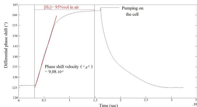
Fig. 3. Detection of hydrogen at high concentration in air.
