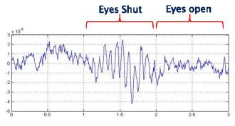
Figure 2. Time domain data showing the alpha blocking phenomena measured using the prototype sensor.
