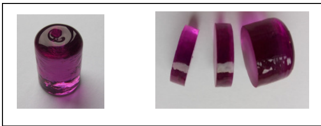
Figure 7. Targets of pH glass
