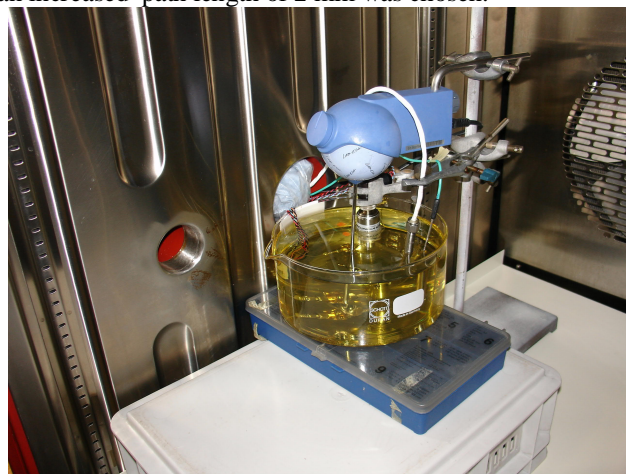
Figure 6. The Hydac, Pal and optical SKF sensors measuring in parallel in a well controlled humidity chamber
