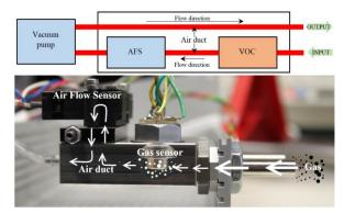
Figure 4. Gas sensor module with air flow sensor and air ducts
