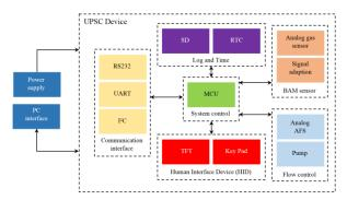
Figure 2. Schematics representation of the functional areas of the system.
