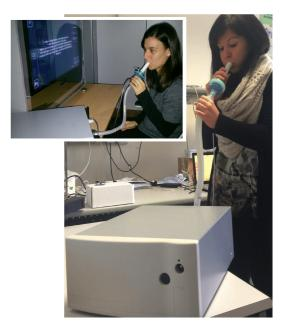
Figure 5. Final configuration of the Wize Sniffer. On the left, the WS is used a Wize Mirror tool. On the right, it is used in a stand-alone configuration.
