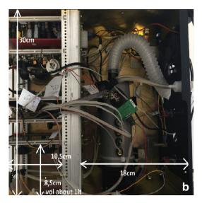
Figure 4. Final set-up of the Wize Sniffer. Internal configuration.
