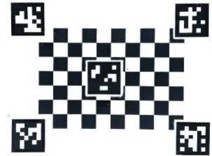
Figure 10. Landing pad with fiducial markers
