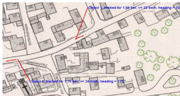
Figure 5. Two trucks have been detected and tracked on a UAV flight. Their velocities and headings can be computed, as in [5].
