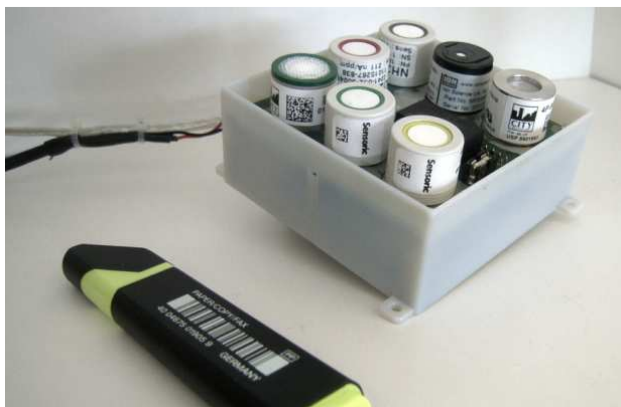
Figure 12. Gas sensor to detect inflammable gases, Ammonia, Nitrogen Dioxide, Sulphur Dioxide, Carbon Monoxide and Chlorine.
