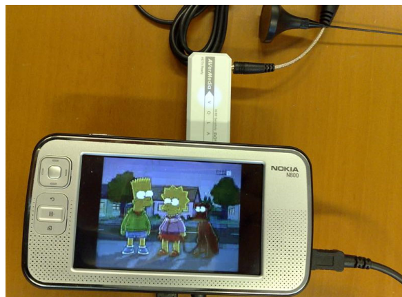
Figure 10: N800 device extended with DVB-H reception.
