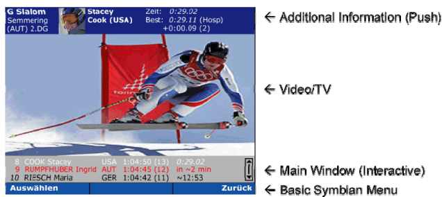
Figure 6: Split-screen Concept for the Mobile TV Client featuring a Live Sports Information service with Push and Pull Content.
