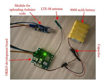
Figure 3. Complete assembly for battery operation.
