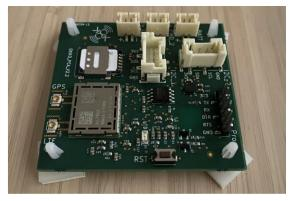
Figure 1. The OKKO board: ESP32-S2 microcontroller + HL7800 LTE-M modem + I2C connectors.
