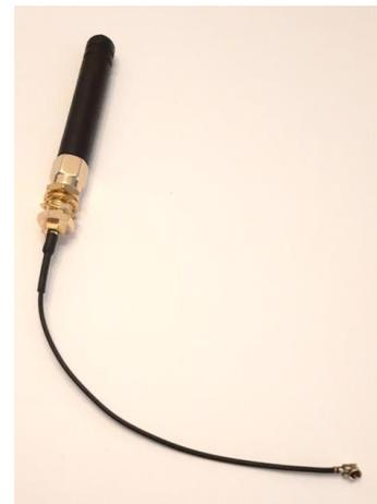
Figure 4. 868 MHz antenna.
