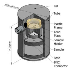
Fig. 2. New design of thermo-formed piezoelectret (TFPA) accelerometer, with polyurethane foam.
