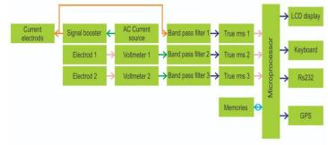
Figure 8. Apparent electrical conductivity system block diagram.
