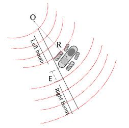
Figure 2. Curved path in which each nozzle has a relative speed which varies according to its position and the curve radius R in relation to the reference point O (figure extracted from [9])
