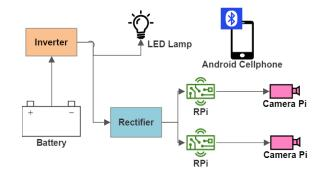
Figure 3. Diagram of the connection between the components.
