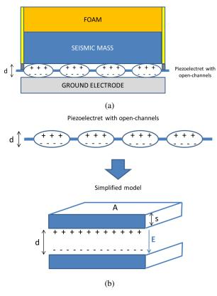
Fig. 4. (a) Cross-sectional view representation of the thermoformed piezoelectret accelerometer. (b) Representation of the simplified model for a piezoelectret.
