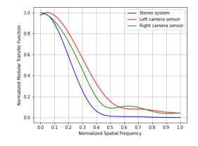
Figure 7. MTF of each camera sensor and combined system.
