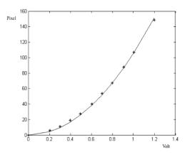
Figure 14. Quadratic behavior between electric power in volt and meniscus' displacement.
