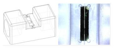
Fig. 5. Left: CAD drawing of the chip housing. Right: 3D printed chip housing with an FBG aligned on top of the  $Si_3N_4$  membrane.
