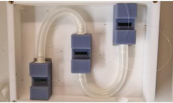
Fig. 6. Measurement device consisting of three cascaded pressure sensors, each on a chip housing, with a single optical fiber.
