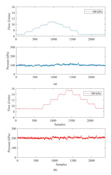
Figure 5. Pressure and flow rates obtained with the valve sequence according to Table III. (a) In the first test the pressure is maintained at 100 kPa. (b) In the second test the pressure is maintained at 200 kPa.
