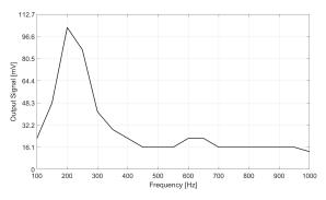
Fig. 6. Frequency response of ADXL327 reference accelerometer output signal peak-to-peak voltage.
