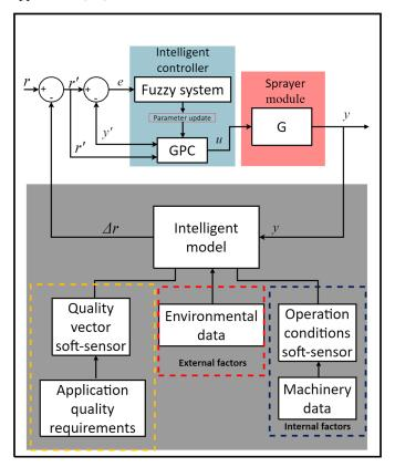
Figure 6. New intelligent control topology for increased quality and efficiency of variable rate application.
