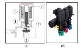
Figure 4. Individual control system for each spray nozzle. (a) Electromechanical system of the solenoid valve (b) Solenoid valves set (model QJS, Teejet<sup>®</sup>) and nozzles (model ASJ WRC, Arag<sup>®</sup>) (Figures adapted from [12])
