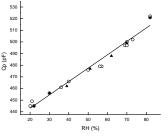
Figure 2. Measured capacitance of a humidity sensor as a function of chamber humidity. (o) measured when humidity was changed ascendingly; ( $\Delta$ ) measured when humidity was changed descendingly.
