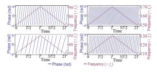
Fig. 2. Frequencies and phases of a multiplexed linear-chirp signal ( $\eta$ =0.05,  $N_f$ =4).
