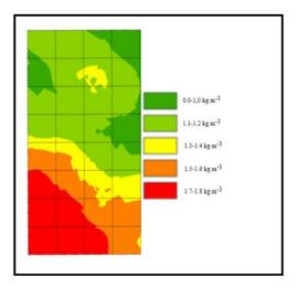
Figure 5. An example of Compton image from the agricultural pilot. The pseudo-color scale is calibrated in (kg.m<sup>3</sup>) and represents the soil compaction presented in the scanned area. From the grid used over the image one may have 25 pixels per block.
