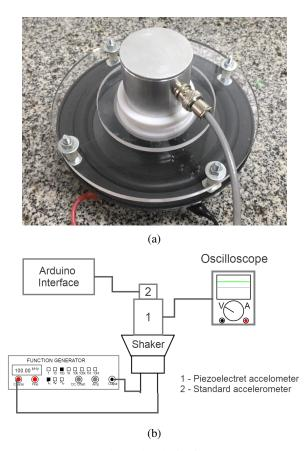
Fig. 3. (a) Custom-made shaker built for the TFPA tests. (b) Block diagram of the experimental setup.
