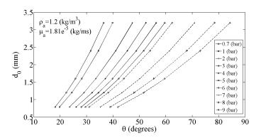
Figure 1. Relationship between the diameter of the nozzle orifice  $d_o$  and the cone angle  $\theta$  for a full cone spray nozzle, simulated for different values of pressure  $\Delta_p$ , for full cone nozzle.
