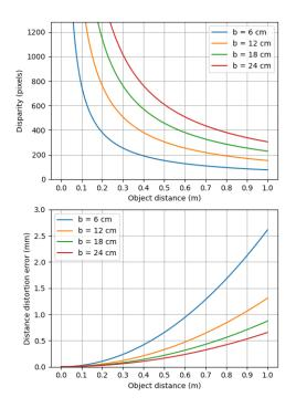
Figure 8. Baseline distance disparity and distortion error evaluation.
