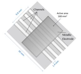
Fig. 1. Sample of Thermo-formed Piezoelectret with channels.
