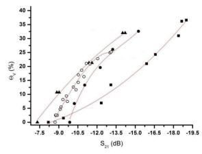
Figure 6. Relationship between the  $S_{21}$  measured with the developed system and the volumetric soil moisture  $\theta_V$  (%). The four (04) samples used are Cerrado Soil (squares), Kaktus Soil (open circles) and Glass Beads (triangles).
