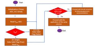
Figure 18. Computational Flow diagram for the real time measurements and flag related to the spray solution pH evaluation.
