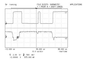
Figure 13. Oscilloscope signal. Above: digitized signal after the voltage comparator. Down: voltage information of the single video line.
