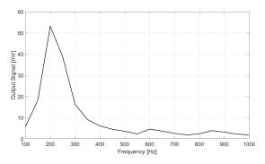
Fig. 5. Frequency response of TFPA output signal peak-to-peak voltage.
