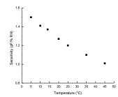
Figure 4. The sensitivity-temperature dependence of a printed relative humidity sensor.
