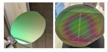
Fig. 4. Left: Wafer with a  $Si_3N_4$  thin film. Right: Wafer with exposed patterns representing the membranes.
