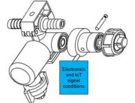
Figure 16. Technical draw of the intelligent pH sensor assembled on the nozzle for direct injection sprayer.
