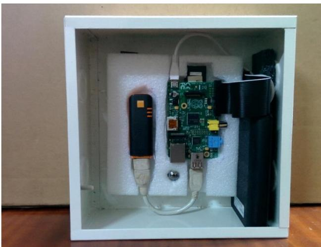
Figure 9. Prototype with Lid removed.
