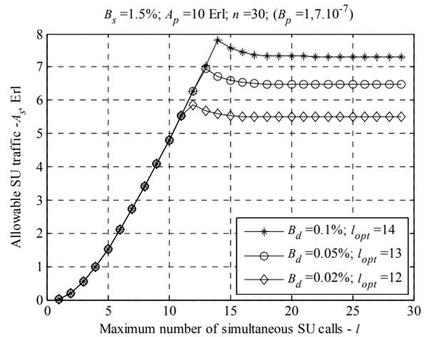
Figure 4. Cognitive VoIP capacity versus the CAC threshold value  $l$  for SU calls.
