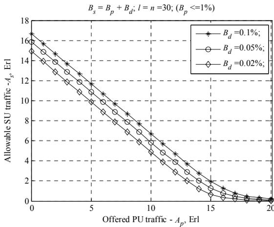
Figure 2. Cognitive VoIP traffic capacity versus the actual PU VoIP traffic load without CAC limitation of SU calls.
