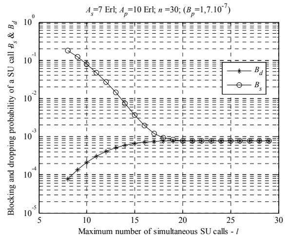
Figure 3. Blocking and dropping probability of a SU call versus the CAC threshold value  $l$  for SU calls.
