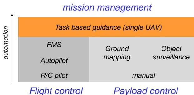
Figure 2. Levels of abstraction in UAV guidance
