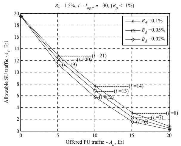
Figure 5. Cognitive VoIP capacity versus the actual PU VoIP traffic load with optimal CAC limitation of SU calls.
