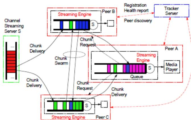
Figure 2. P2P streaming process [8]
