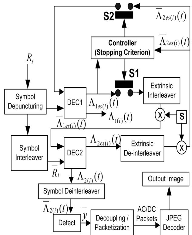
Figure 2. Decoding system with enhanced duo-binary Decoder.
