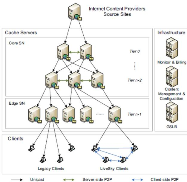
Figure 3. System architecture
