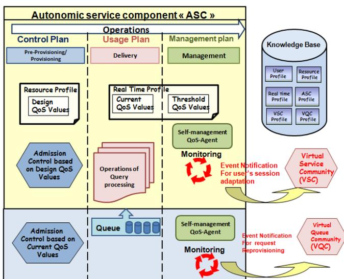
Figure 2: QoS Management Mechanisms applied by the ASC
