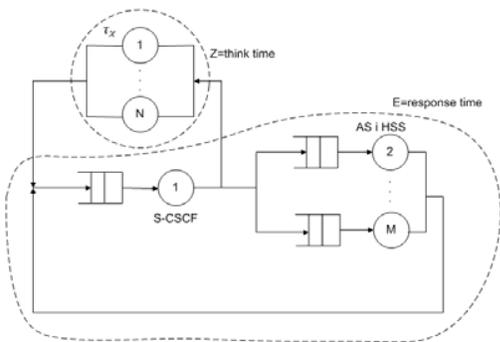
Figure 1. Model of central server for IMS [2]
