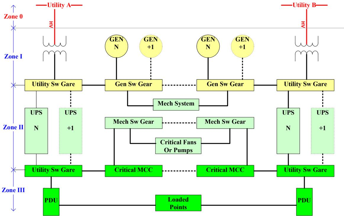
Fig. 1. Original Tier IV Data Center Diagram [3]
