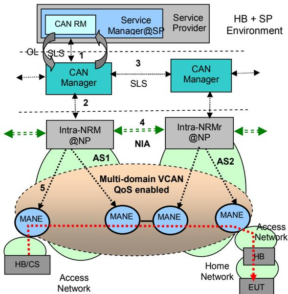
Figure 1. High level ALICANTE architecture: multi-domain VCANs and main management and control interactions
