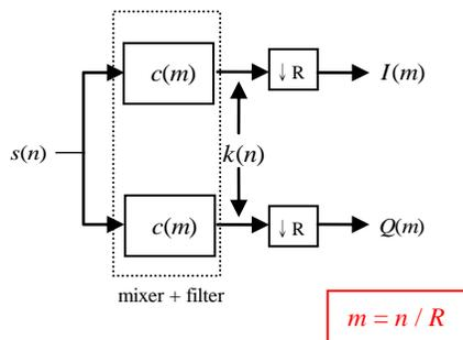
Figure 6. The block diagram of proposed *CMF*
