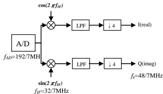
Figure 4. Digital-Down-Converter using  $f_s = 192/7$ MHz
