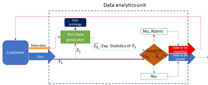
Fig. 8. Feature selection and decision making procedure in more details for the third solution.
