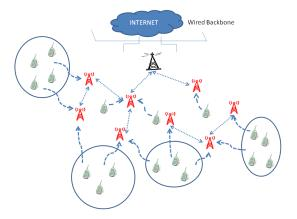
Fig. 1. Multihomed MCN where sets of user nodes are connected to a home relay and home relays communicate with other home relays in its transmission range to transmit information to the base station
