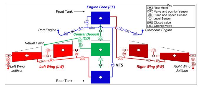
Figure 5. Physical illustration of aircraft fuel system.
