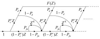
Fig. 2. A generation function flow graph of the acquisition schemes based on the sequential estimation.
