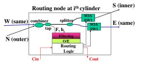
Figure 2. Routing node implementation
