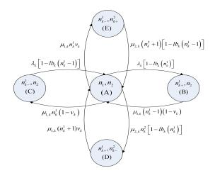
Figure 2. State transition diagram of the OCDMA system with active and passive users.
