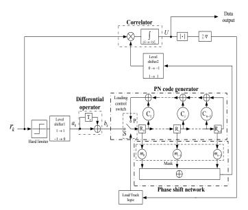
Fig. 1. A structure of the PDSE receiver.
