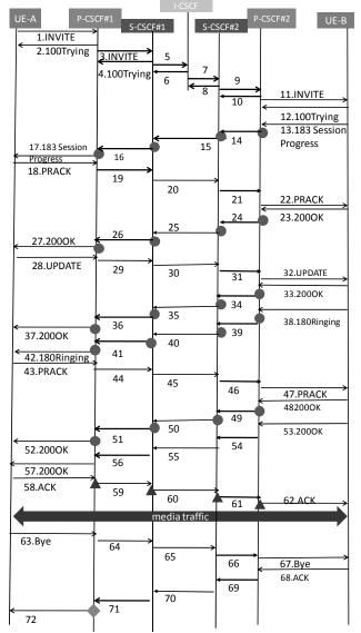
Figure 3 Application initiation procedures of IMS
