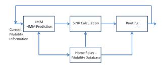
Fig. 2. Block diagram that illustrates the interaction between the LMM model and the interference aware routing algorithm
