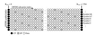
Fig. 1. Pilot arrangement in a DVB-T system with 2K mode.
