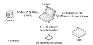
Figure 2. Overview of the infrastructure of the system setup, including description of data
