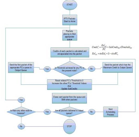
Figure 4. Flowchart of the Proposed Algorithm
