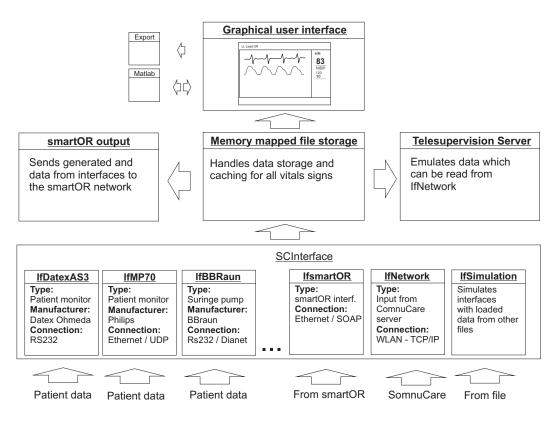
Figure 4. Functional diagramm of SomnuCare
