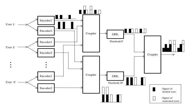
Figure 1. Block diagram of the transmitter of the proposed system.
