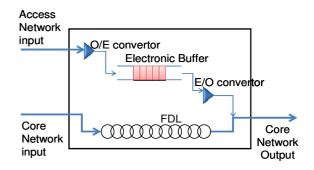
Figure 2. Architecture of Hub
