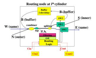
Figure 4. Routing node with buffer implementation: a 2-slot delay for buffer path is necessary to setup the control signal on time and additional controls  $C_{out2}$  are used to inform the state of buffer
