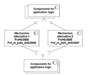
Figure 3. Component diagram after reliability predictions
