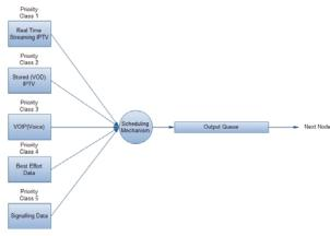
Figure 1. Priority Based Classified Scheduling Node Structure
