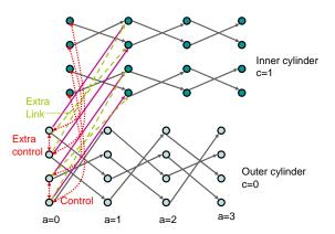
Figure 5. Additional inter cylinder path in Data Vortex network with required extra control
