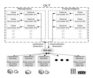
Figure 1. A basic configuration of an OCDMA PON
