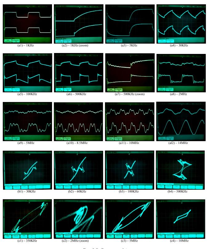
Figure 8. Oscilloscope screenshots. (a) Voltage responses on 2 different pins with input square wave at different frequencies. (b) XY plots, X (OUT1) is plotted against Y (OUT2) at different frequencies. (c) XY plots, X (IN) is plotted against Y (OUT1) at different frequencies.
