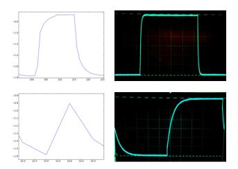
Figure 5. Mecobo (left) vs. oscilloscope (right) at 1KHz (top) and 10KHz (bottom). Input ±3.3V, duty cycle 50%.
