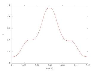
Figure 5. The course of the state variable x of a memristor cell
