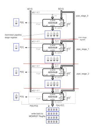
Figure 8. Memristor-based pipelining for the multiplication of a SD number, a, and a binary number B
