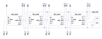
Figure 6. Schematic for a 4-digit SD adder that can add/subtract a SD number a and a binary number B
