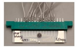
Figure 2. Electrode array slide plugged into connector.
