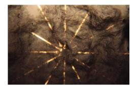
Figure 7. SEM image of gold electrode arrays with different coverage of nanotubes. Adopted from [8].
