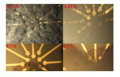
Figure 2. Optical micrographs of SWCNT-polymer nanocomposites dispersed over gold electrodes with  $25\mu m$  electrode gap. Different concentrations exhibit various coverage of gold electrodes.
