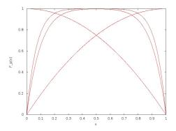
Figure 2. Modelling non-linearity with Biolek's window function for different parameters p = 1, 5, and 7. Considered is also I(t) < 0, the curve starting at  $F_p(0) = 1$ .
