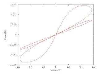
Figure 4. The memristor hysteresis loop, generated for D = 41nm, x(0) = 0.11, and p = 7. For each excited voltage oscillation another hysteresis behaviour is generated
