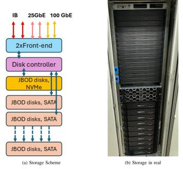
Fig. 2. Architecture of the storage subsystem (replicated each 2.5 PBytes)
