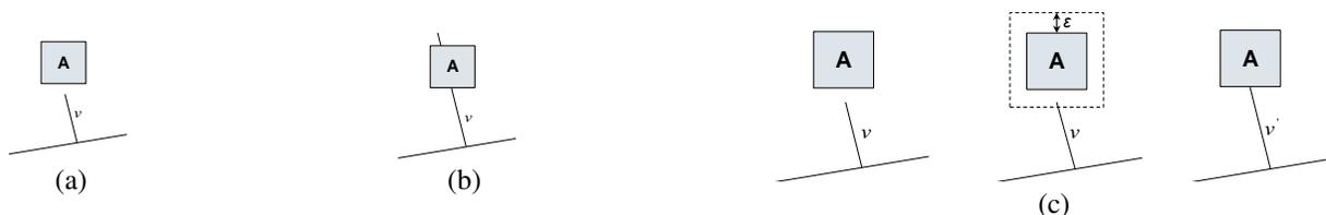
Figure 2. Dangling lines: a) undershoot, b) overshoot, c) correcting dangle using a tolerance gap
