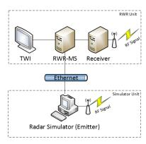
Figure 5. System Components
