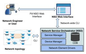
Figure 3. Architecture used in the proposal
