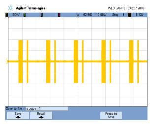
Figure 6. Radar Simulator Output (Oscilloscope Screen)
