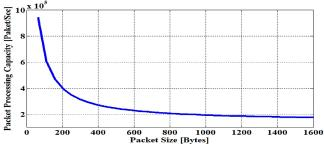
Figure 7. The relation between packet processing capacity and packet size.
