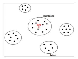
Figure 1. Example of an Island-Based WSN.
