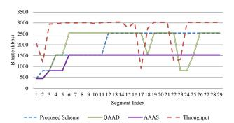
Figure 3. Comparison of the schemes in response to large throughput fluctuation
