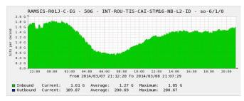
Figure 2. (a) Daily traffic profile of core TE Data network router peering with TIS.
