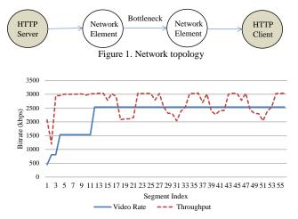
Figure 2. Response of the proposed scheme to small drop in throughput
