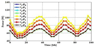
Figure 4. Power consumption of packet processing according to various configurations of P-and C-states.
