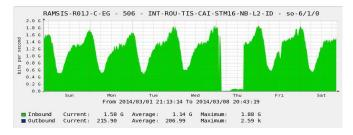
Figure 3. (b) Weekly traffic profile of core TE Data network router peering with TIS.
