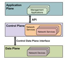
Figure 1. Logical structure of SDN
