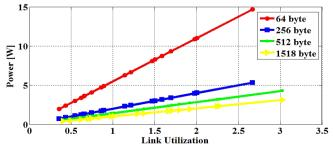
Figure 6. Power consumption of router interface with different packet size.
