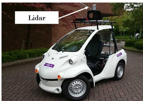
Figure 1. Overview of the experimental vehicle.
