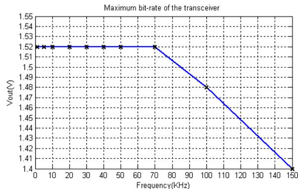
Figure 6. Maximum possible bit-rate of the transceiver
