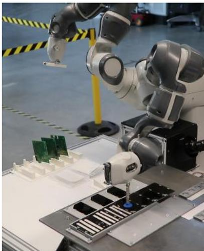
Figure 3. Robotic assembly of a satellite solar array.
