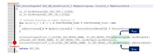
Figure 4. View of the core function of ASC. At the position of the selected breakpoint, the input matrix  $x_{HW}$  and the associated output matrix  $y_{HW}$  for the diagnostics from the hardware can be read.
