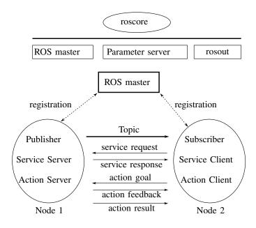
Fig. 2. ROS core communication system, and different message communication modes between nodes (adapted from [17]).
