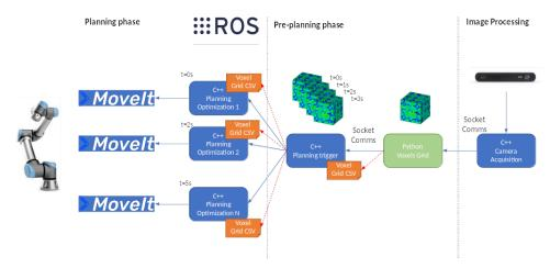
Fig. 3. Path planning solution architecture and module relationship.
