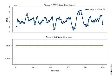
Figure 5. Evaluation diagram with 100 iterations of the diagnostic loop for the Sensor Tile diagnosis system.
