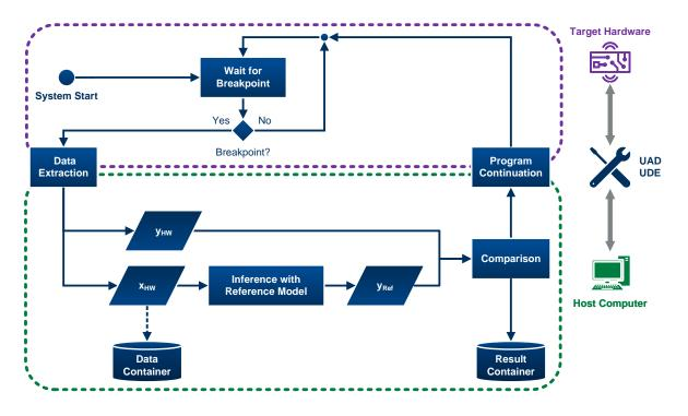
Figure 2. Schematic structure of the diagnostic loop for the continuous comparator-based analysis of the hardware and model outputs. Purple dashed frame: Processes belonging to the context of the target hardware. Green dashed frame: Processes belonging to the context of the host computer.
