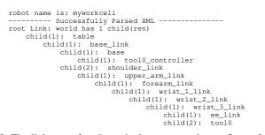
Fig. 5. The link tree of UR5 manipulator mounted on a flat surface 'table'.
