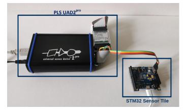
Figure 3. STM32 Sensor Tile connected to the PLS UAD2pro.
