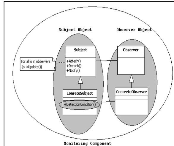
Figure 1. Monitoring Component in the logical layer
