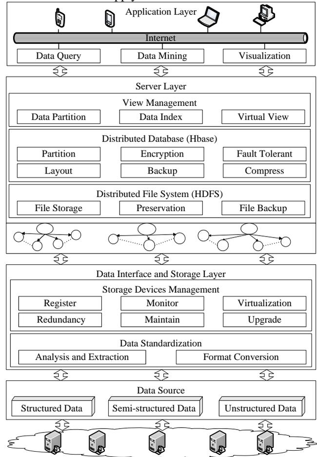
Figure 2. Cloud platform architecture
