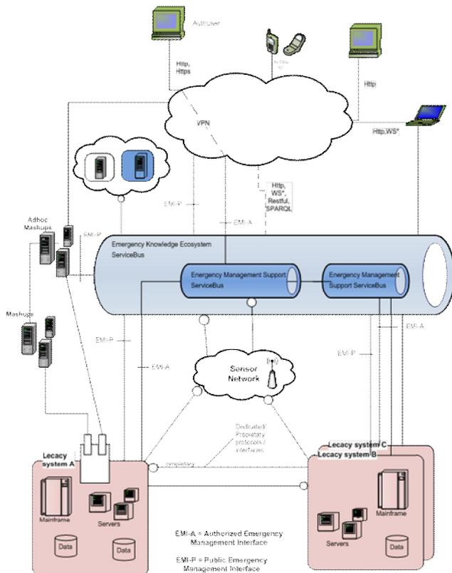
Figure 3. Service-oriented system architecture for Emergency Management Knowledge Ecosystem [6]
