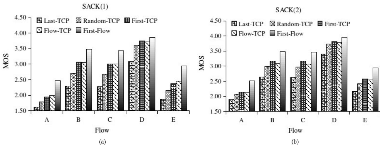
Figure 3. E-MODEL based MOS evaluation of dropping policies.
