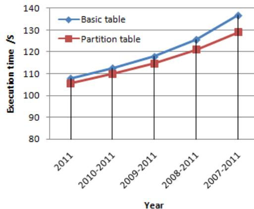
Figure 7. The query execution time of partition table and basic table
