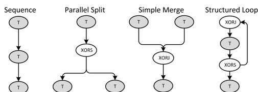
Figure 5. Query CFP represented through logical gates
