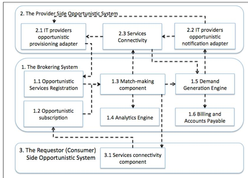
Figure 1: Conceptual architecture of a community-commerce brokering system
