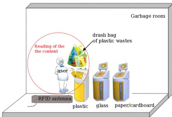
Figure 11. An individual bin using the RFID technology.
