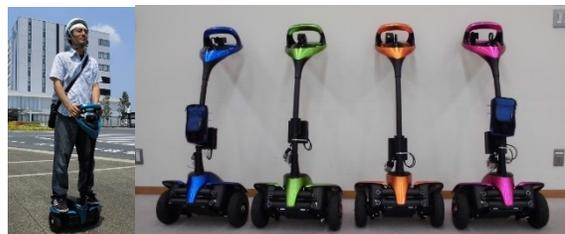
Figure 2. Winglets (equipped with mobile sensors)
