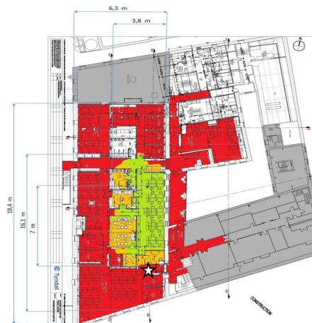
Figure 8. Bluetooth range test
