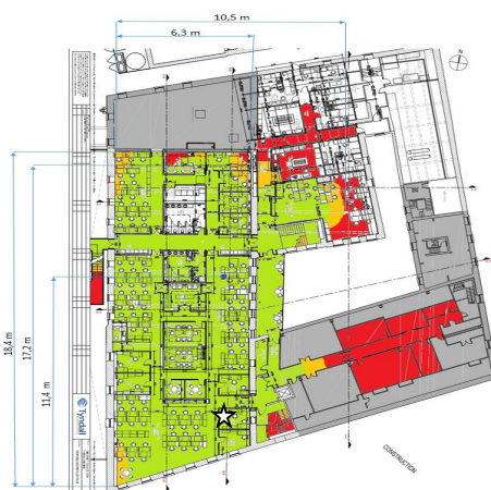
Figure 7. 868MHz range test
