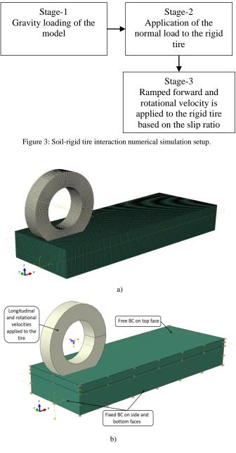
Figure 4: a) CEL model discretization b) CEL model BC.
