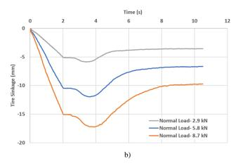
Figure 6: a) Net Traction performance b) Tire Sinkage (Slip ratio-18.5%).
