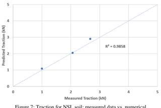
Figure 7: Traction for NSL soil: measured data vs. numerical predictions [10].
