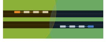
Fig. 2. Representation of offloading intra-platoon communications to RadCom. The yellow and blue shades represent the coverage area for the members of each platoon, yellow for the westbound and blue for the eastbound.
