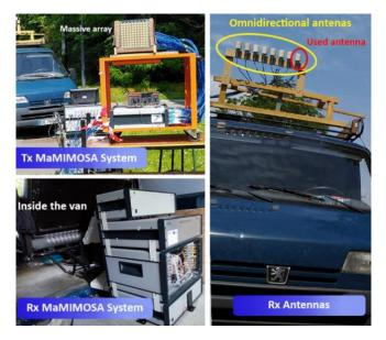
Figure 2. Tx-Rx antenna systems.
