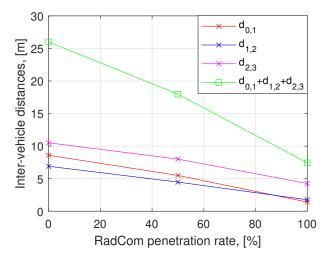
Fig. 3. Safe inter-vehicle distances in a platoon of four vehicles versus RadCom penetration rate. Here,  $d_{i-1,i}$  denotes an inter-vehicle distance between vehicles i - 1 and i where vehicle 0 is the leader.
