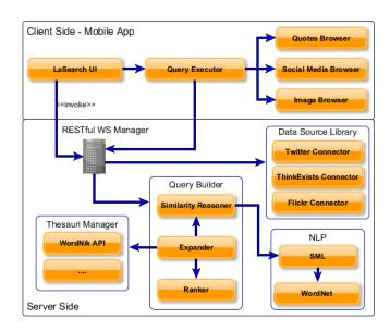
Figure 3. Architecture of the implemented prototype
